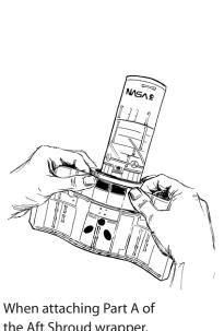
When attaching Part A of the Aft Shroud wrapper, make sure that the NASA logo on the Forward Shell and the three circular shapes on the Aft Shroud Part A form a straight line.
